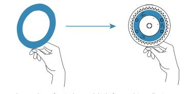
1.Make sure the surface is clean and dry before applying adhesive. 2.Apply the included 3M double-sided tape to the bottom of the controller. 3.Remove the other backing. 4.Press the device firmly with both hands for 30 seconds to secure it in place. 7
